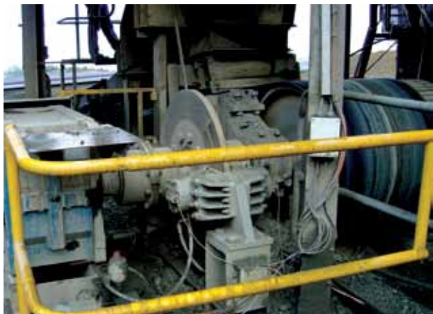
Twiflex VKSD spring-applied hydraulic released brake units fitted on copper mine conveyor in Tasmania, Australia.
