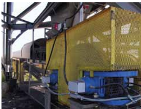
Twiflex VS180 spring-applied hydraulic released brake units fitted to an overland coal conveyor in West Virginia.
