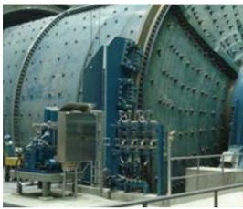
*Twiflex VMS-DP brake calipers (with pedestals) plus a hydraulic power pack installed on a 22.5 MW SAG mill, 11.6 m dia. x 13.7 m long, at a copper mine in Sweden. The 8-off VMS-DP brakes produce 38 MNm braking torque and can stop the mill with the 1375 Mg full process charge in less than 2 seconds.*
