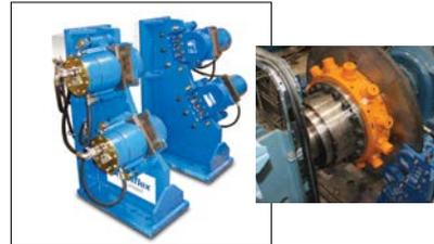
*Pairs of Twiflex VKSD-FL brakes (with pedestals) for installation on a 24 ft. dia. dual-pinion, direct-drive geared ball mill at a copper/gold mine in Canada. The VKSD-FL (floating) calipers act on a brake disc fitted to a torque limiter. The brakes provide 454 kNm on the mill's high-speed shaft.*
