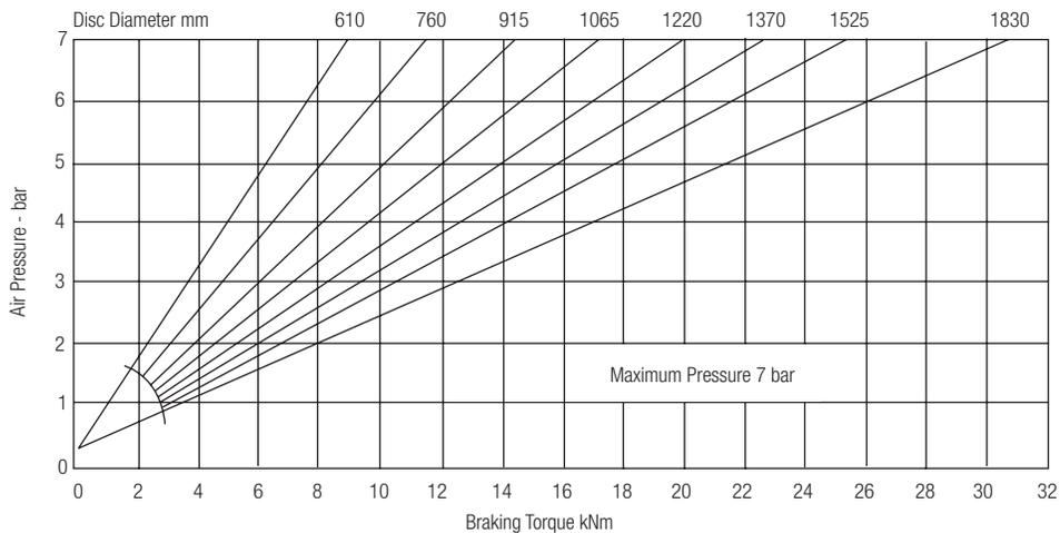
Maximum Braking Force = 36kN
